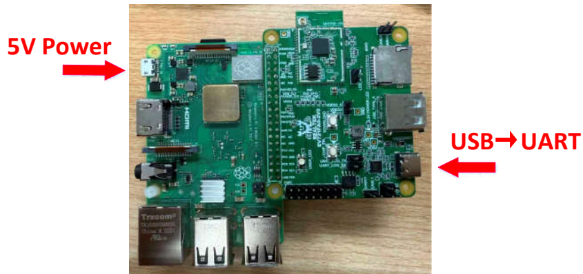
Figure 4-11 Power supply method of the system
