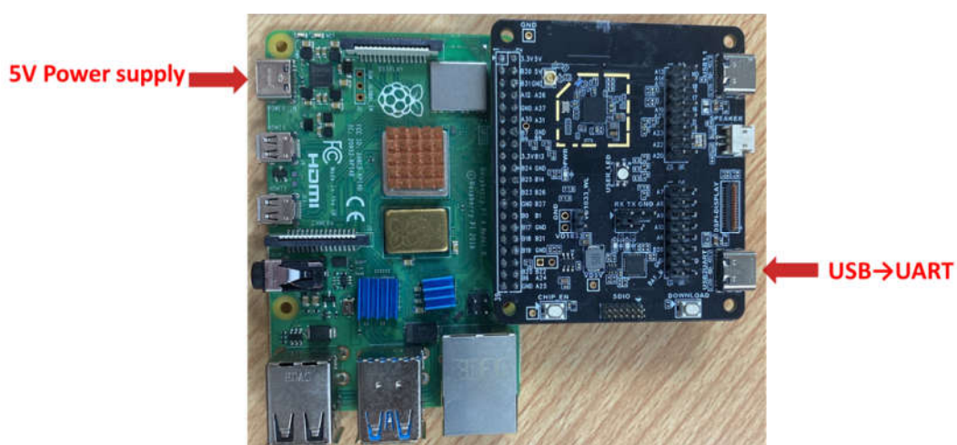
Figure 4-6 Power supply method of the system when EVB preforms as slave
