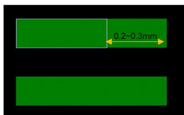
Figure 14-4 Length of outer lead perimeter size to the package edge
