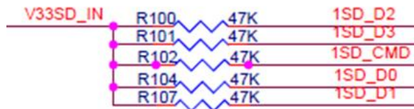
Figure 12-3 PULL-UP resistors for SD signals
